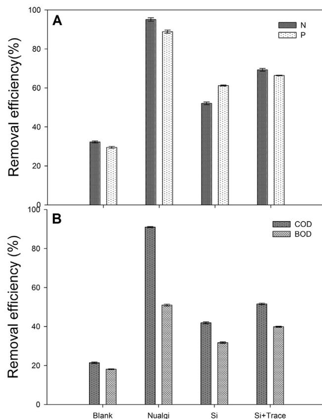
**Fig. 2.** Total nitrate (TN) (A), Total phosphate (TP) (A), Chemical oxygen demand (COD) (B) and Biological Oxygen Demand (BOD) (B) reduction from waste water by Diatom consortium under different Nutrient enrichments. Bars indicate SD.
